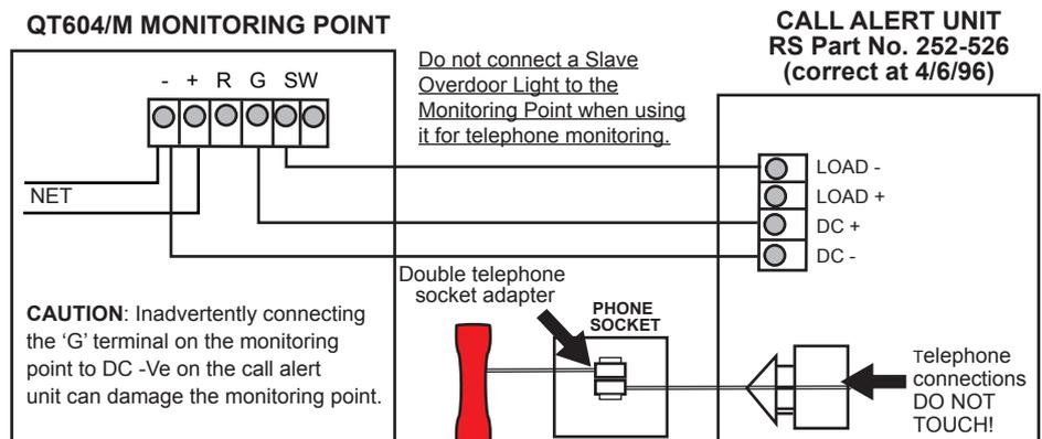
These instructions only apply to Monitoring Points with the legend Rev3 or later, on the PCB. Alternative instruction sheets are available for earlier versions. Contact your supplier for details.
